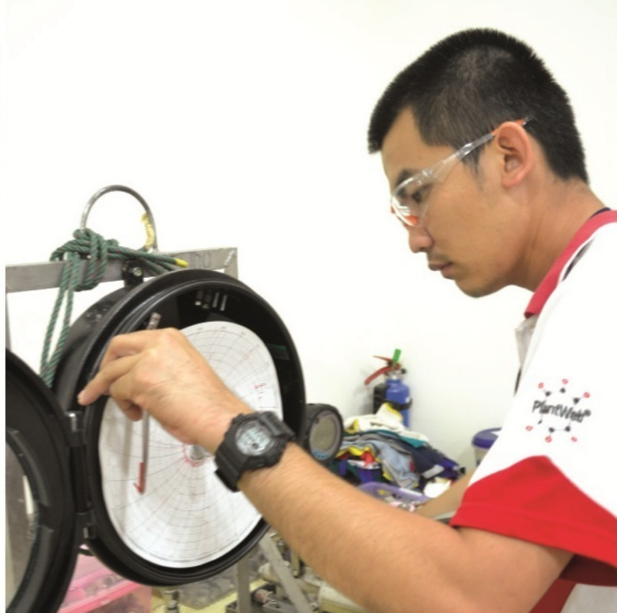
■ Well-trained technician performing a pressure recorder calibration.
